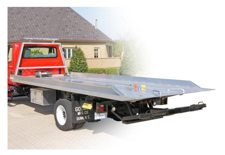
True rollback carriers Godwin car carriers are true rollback carriers available in lengths of 18', 19' and 21', using 5" bronze bushing rollers. It has unique features like the patented Godwin rollback locking system, which automatically locks the bed to the truck when in the down position. It automatically unlocks when the body tilt hydraulics are activated.
