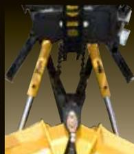
Put the plow in any configuration, and lock it into position with the standard locking double-acting cylinders. You can plow or back drag with ease; just set the angle you want, and you're ready to plow.
