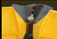
An exclusive upper-sealed center deflector and optional wing deflectors keep snow and ice off your windshield. The standard lower-sealed center deflector never leaves snow trails behind, so there is no mess to clean up after using your V plow.
