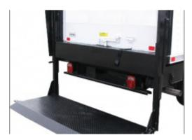
The RCM offers unique flexibility and lifting capacities up to 1600 lbs for your van body, cutaway, step van, platform or stake body.
