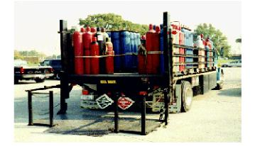
This Thieman VLBG Series is designed for handling gas bottle cylinders. Like the VL series, it is built with the strongest, most durable frame in the industry. The VLBG also incorporates high quality roller bearings and cycle tested, premium lift cables for smooth operation.
