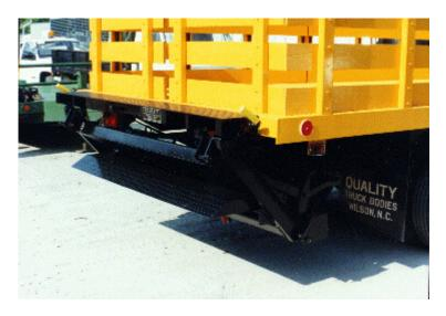
The Thieman LST Series is designed for use on stake and van bodies and trailers. The *outside lift arm* design gives the operator maximum stability when handling sizable loads.
