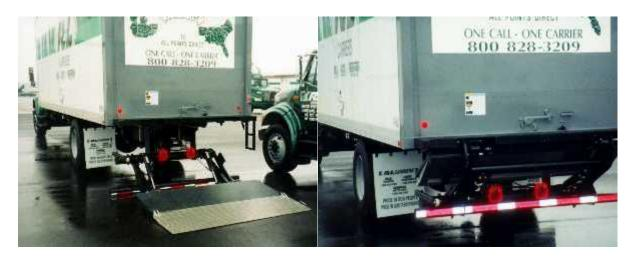
The Thieman ST Series is a premium, *heavy-duty* Stowaway designed for use on heavy-duty trucks and trailers. With the exception of the ST-22, the entire ST Series incorporate a dual cylinder lift for maximum lifting strength and stability.
